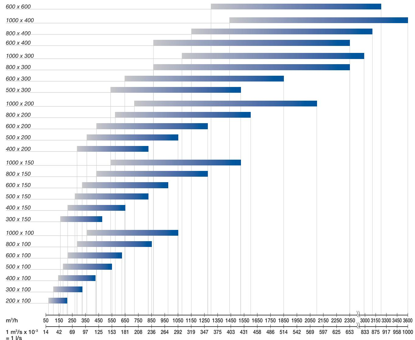
The air flow rates and the pressure drop rates are certified according to the UNI 8728 and prEN 12238 standards, by an independent and certified body, in compliance with the legislation in force on energy saving standards.
